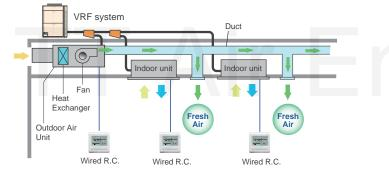
\* Make sure the connected capacity is within the range of 50% to 100% of the outdoor unit capacity. In addition, if there are mixed connections with indoor units, make the Outdoor Air Unit connection capacity 30% or less of the outdoor unit capacity.
