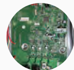
3 Sine-wave DC inverter control
