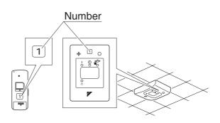
Operate the indoor unit with the remote controller of the same number.
