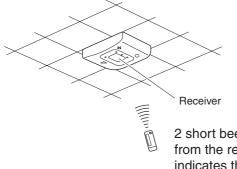
2 short beeps from the receiver indicates that the transmission is properly done.
