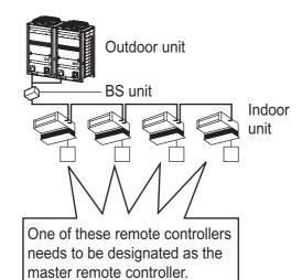
Only the master remote controller can select HEATING, COOLING or AUTO-MATIC (only Heat recovery system) OPERATION.
