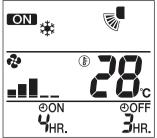
When the timer is programmed to stop the system after 3 hours and start the air conditioner after 4 hours, the air conditioner will stop after 3 hours and then 1 hour later the air conditioner will start.
