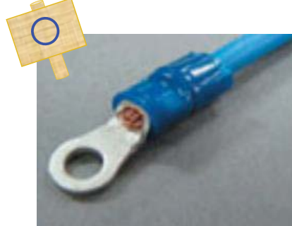
Crimped using an appropriate tool
