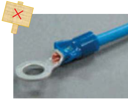
Crimped using a tool for bare crimp-style terminals
