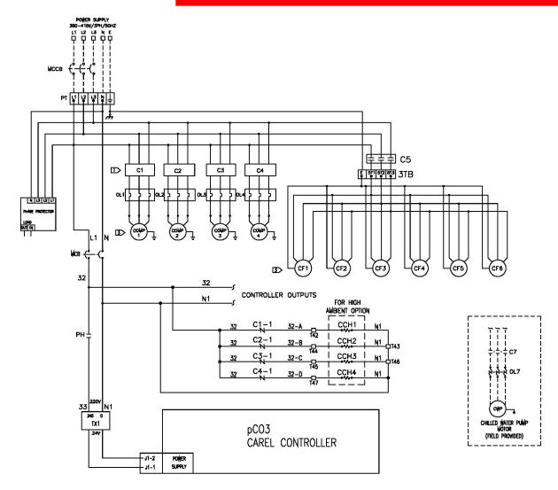
NOTE :-FOR CGAPO60 - COMPRESSOR OVERLOAD ARE INTERNALLY PROTECTED
