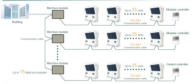
The unit can be connected to the building management (System BMS) by the standard Mod Bus communication protocol, which can support up to 375 units.
