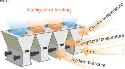
• When modular connected, the master controller will calculate and balance the defrosting time of each module automatically. The defrosting operations in any modules will not impact the normal working of the others, so as to guarantee the continuous heating in winter.
