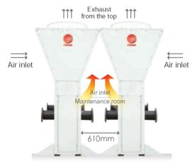
It is suggested to put the unit at a place with good heat dissipation and at least 1.2m away from the wall.
