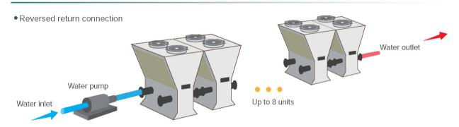
Note: For multi modules, up to 8 units in single module. Direct return connection is not allowed.
